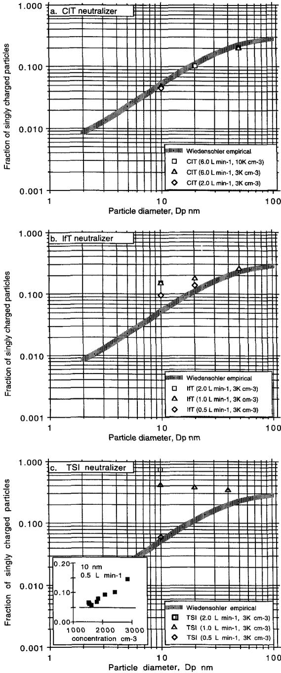
FIGURE 4. Particle charging efficiencies for three neutralizer designs. Data points are the experimentally determined values and lines are the theoretically predicted fraction of charged particles according to Wiedensohler (1988). The inset in the graph of the TSI data (c) shows the measured concentration dependence of recharging.
