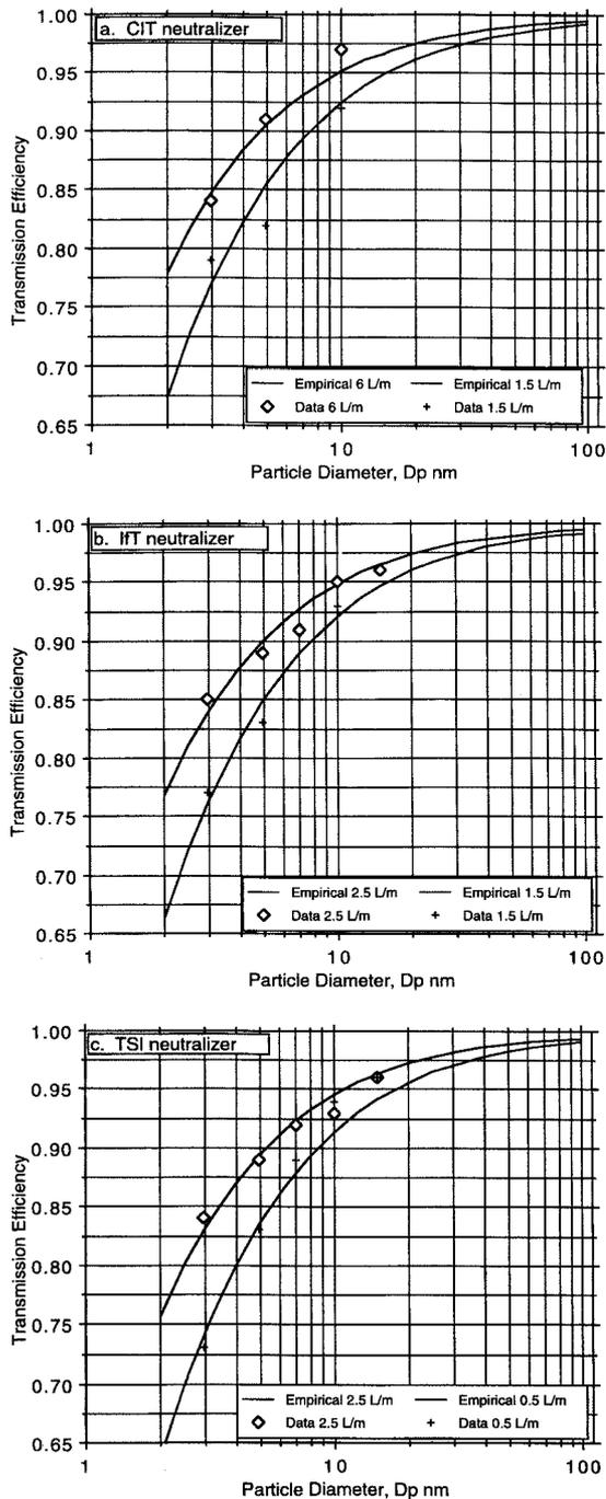
FIGURE 2. Transmission efficiency for three neutralizer designs. Data points are experimentally determined values and lines are the calculated values from a least square fits to data using an exponential equation of the form of Gormley and Kennedy (1949).
