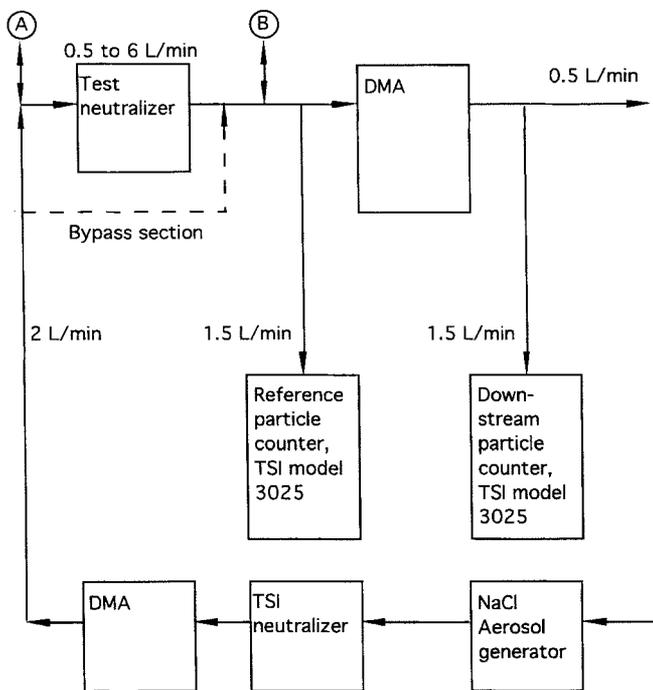
FIGURE 3. Schematic of experimental apparatus for recharging efficiency tests. Points labeled A, B, and C indicate sources and/or sinks of air used to balance flows through the various components of the system.
