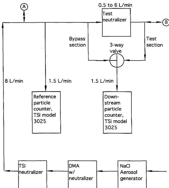
FIGURE 1. Schematic of the experimental apparatus for particle loss tests. Points labeled A, B, and C indicate sources and/or sinks of air used to balance flows through the various components of the system.
