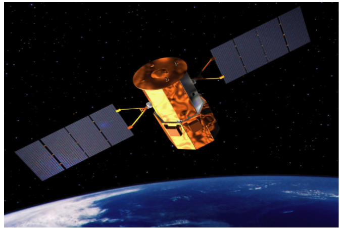
Fig. 3: NASA Glory Satellite to be launched in December 2008. Onboard instruments will include the Total Irradiance Monitor (TIM) and Aerosol Polarimetry Sensor (APS).
