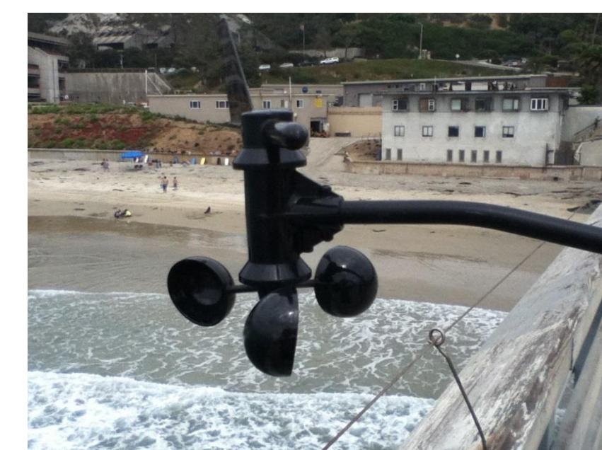
Wind speed and direction anemometers
