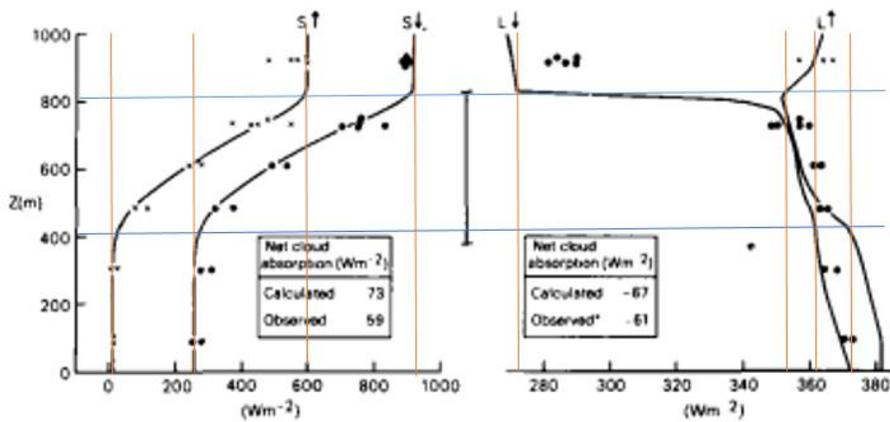
Figure 2 Longwave radiation balance from Nicholls (1984). The blue lines represent the cloud top and bottom. The orange lines represent the flux values.
